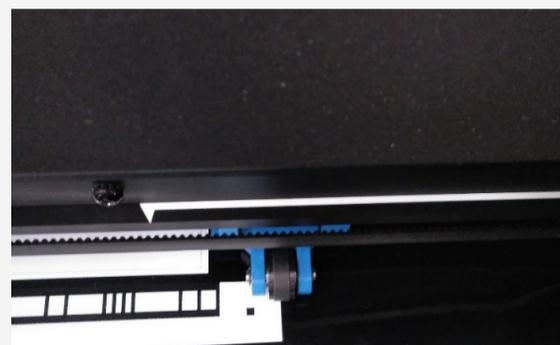
Position the plot so that the first pinch partly rolls over the white part of the HP barcode (see picture).
